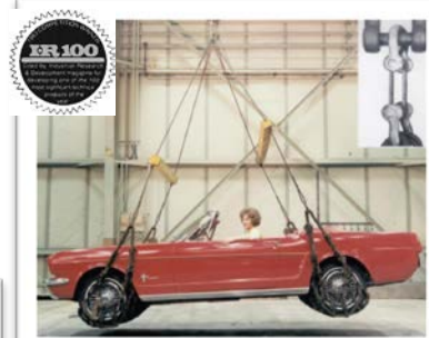
August 1966 3000 lb Mustang supported by a loop of carbon fiber reinforced resin
